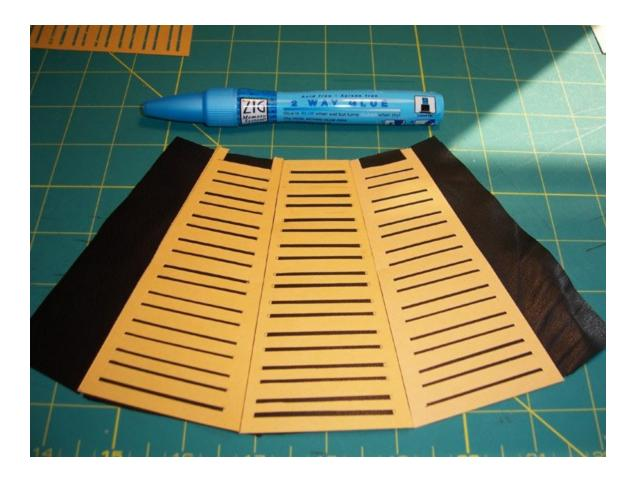
8. Now you need another template. This is best described as a pyramid with a flat top. The sides are the same measurements as the template shown in Step #2. They are made a little longer at the base so that it is easier to work with (you can see a line toward the bottom of the structure. That is where the bellows ends). I made this out of 4-ply photo mounting board and packaging tape. Be sure to make an insert at the bottom and top to make the structure rigid.
