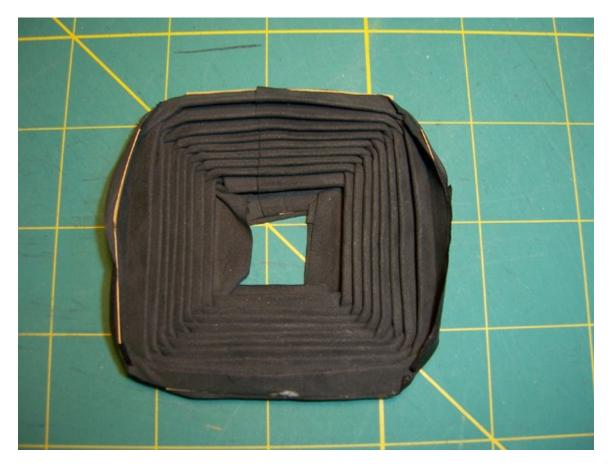
21. The next step is to mount the brass front plate, but first we need to look at the trimming of the bellows for mounting. Even though our bellows was constructed with equal length sides, as you can see in the following picture of a bellows removed from a camera, the first fold of the front portion of two of the sides has been removed. This is because the mounting of the bellows on the front plate (and also on the back portion at the film plane) has to result in adjacent folds being opposite.
