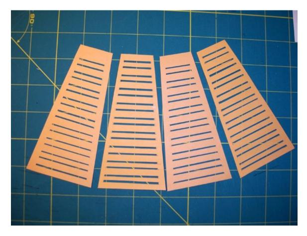
Then I cut the finished sheet into the four pieces. In the picture above, rib structures 1 and 3 (from the left) are for the sides and rib structures 2 and 4 are for the top and bottom.
