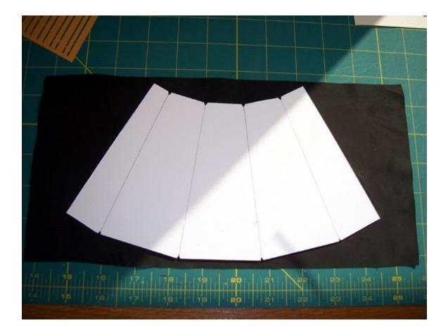
For both the liner and cover I use a very thin leather (.007") that I can get in sheets that are 6" x 12" which is a good size for these bellows.
