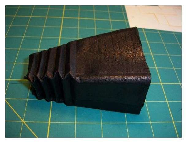
19. At this point I place the bellows face down on my work table and begin folding from the back. It is easier for me to do it this way since I can see how the folds need to occur and also allows me to use both hands to fold and push down on the table.
